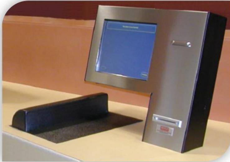
The Sentry RFID QuickCheck™ (Model QC5) provides patron checkout and renewals of materials via RFID tags and barcodes. When the RFID tag or barcode is read, an EAS/AFI security function is performed, the items are processed, and a receipt is printed informing the patron when to return materials to the library.
